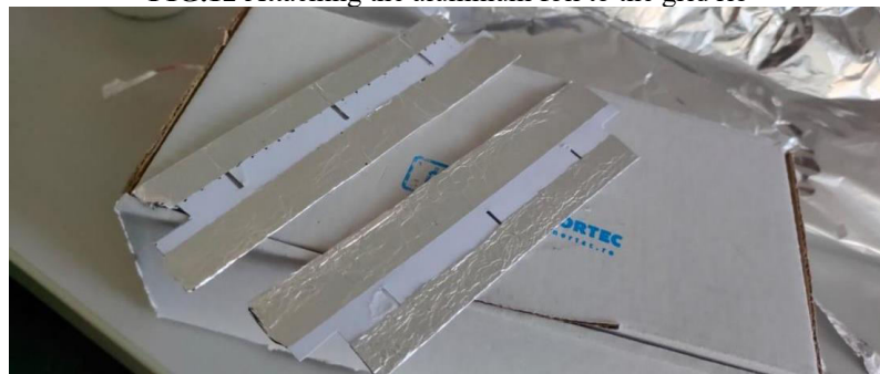
FIG.13 Grid ribs with aluminum foil attached
