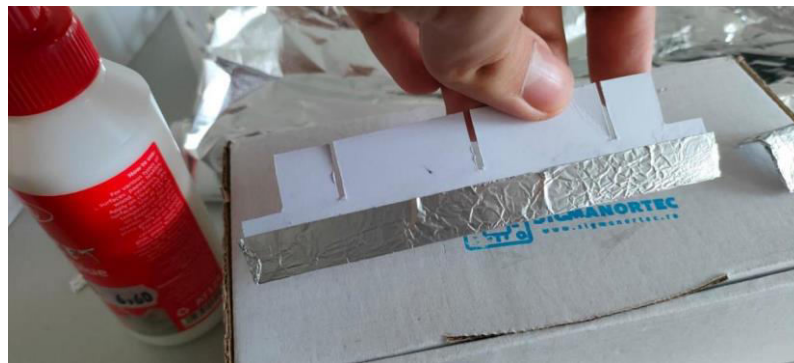
FIG.12 Attaching the aluminum foil to the grid rib
