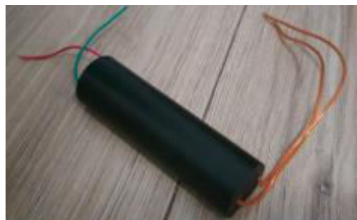
FIG. 2 High-voltage generator module (1000 kV output, 3–6 V input), used in ionic propulsion experiments.
