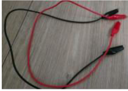
FIG. 3 Alligator clips (crocodile clamps) used for temporary electrical connections in the test circuit.
